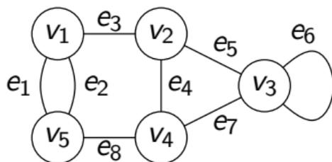
$$B(G) = \begin{matrix} & e_1 & e_2 & e_3 & e_4 & e_5 & e_6 & e_7 & e_8 \\ \begin{matrix} v_1 \\ v_2 \\ v_3 \\ v_4 \\ v_5 \end{matrix} & \begin{pmatrix} 1 & 1 & 1 & 0 & 0 & 0 & 0 & 0 \\ 0 & 0 & 1 & 1 & 1 & 0 & 0 & 0 \\ 0 & 0 & 0 & 0 & 1 & 2 & 1 & 0 \\ 0 & 0 & 0 & 1 & 0 & 0 & 1 & 1 \\ 1 & 1 & 0 & 0 & 0 & 0 & 0 & 1 \end{pmatrix} \end{matrix}$$
